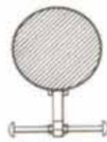
Overhead View Step Hole Aligned Ladder Feet Pegs are Aligned for Easier Climbing
