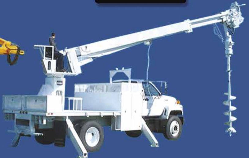
CHEVROLET Diesel Texoma TX-245B Digger Derrick
